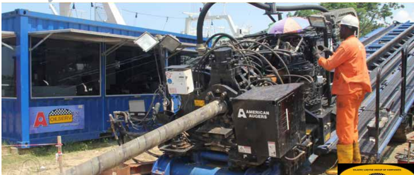
• Oilserv HDD equipment ready to undertake a major river crossing operation
